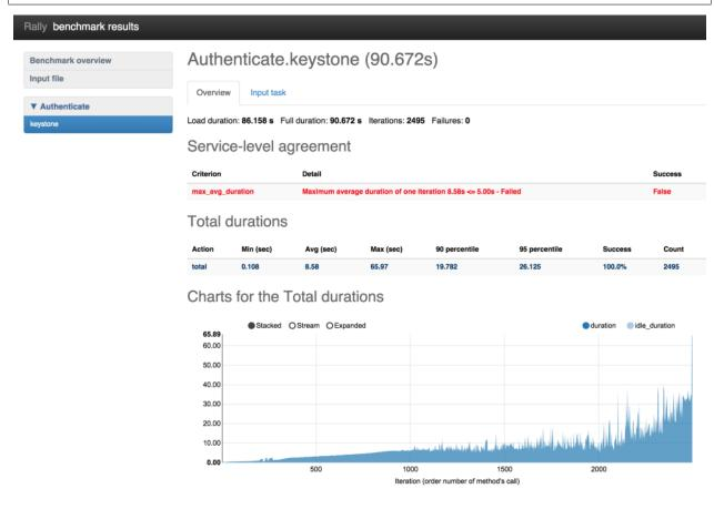
On the chart with durations we can observe that the duration of authentication request reaches 65 seconds at the end
