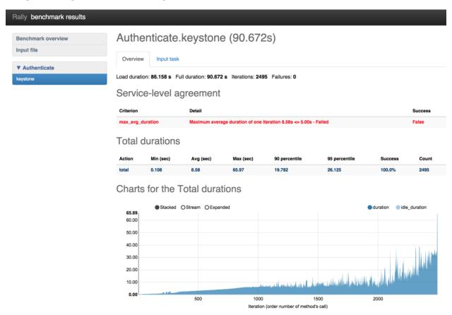
On the chart with durations we can observe that the duration of authentication request reaches 65 seconds at the end of the load generation. Rally stopped load at the very last moment just before the mad things happened. The
